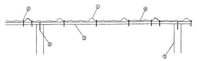
1. Metal Roof Deck Panels\* — No. 29 MSG min. thick coated steel. 36 in. wide (cover width).
